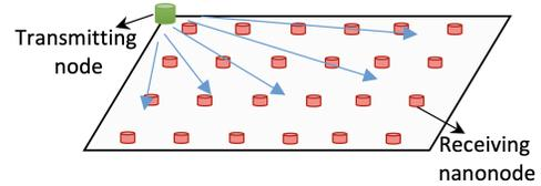
Figure 2: Envisioned grid-like constellation of receiving nanonodes with a single transmitting node
