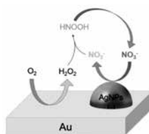
Figure 1: Mechanism of electroreduction of nitrate ions on a modified gold electrode
