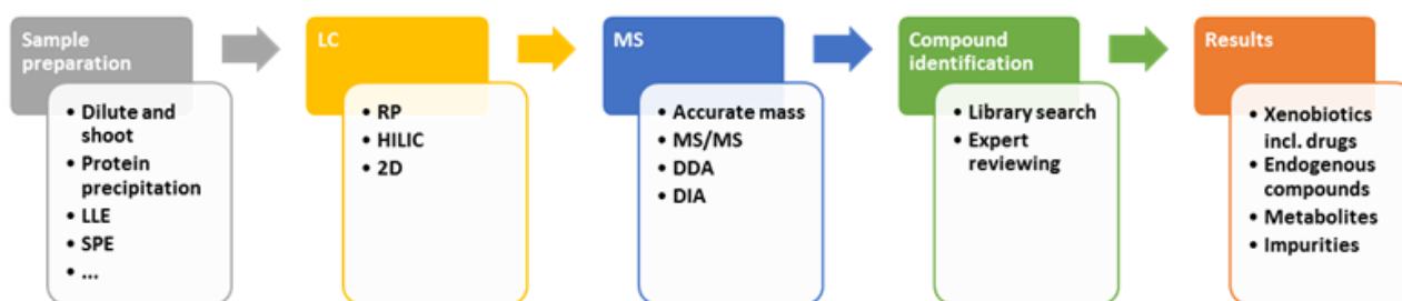
Figure 1: Non-target/suspect screening workflow. Adapted from Oberacher et al. [3,4].
