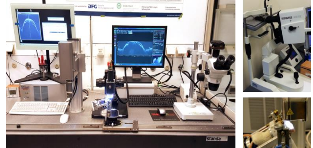
Left: HSM and Telesto (high resolution OCT & fluorescence imaging), Right-top: HRA-OCT (clinical retinal OCT), Right-bottom: Animal holder
