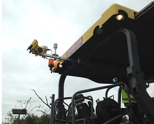
infrarood linescanner (Pave-IR Moba)
