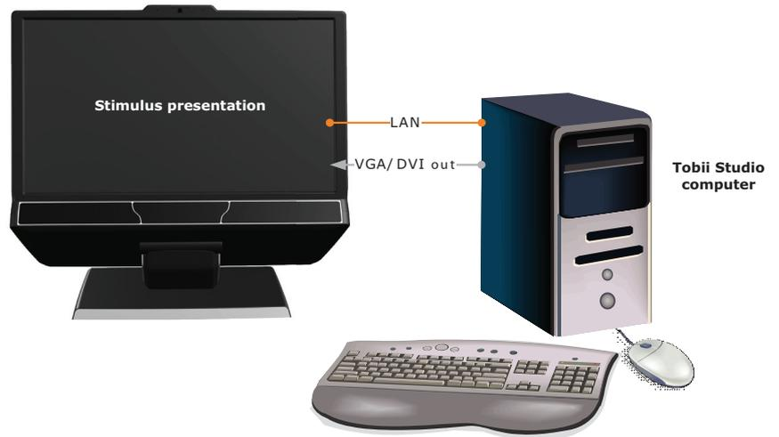
This basic setup is the simplest setup when using on-screen stimuli, such as images, movies, web or software. The image above illustrates the single screen setup. The eye tracker is connected to the computer via the computer's LAN connector and a VGA or DVI cable. To create a portable lab, replace the computer in the setup drawing with a laptop or shuttle computer.
