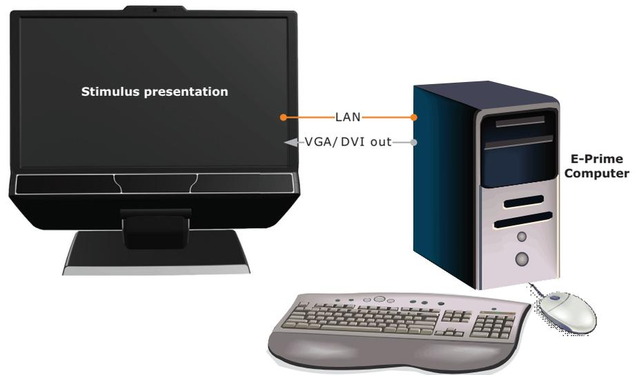
The E-Prime® software and Tobii Studio software are run on the computer and communicate with the Tobii Eye Tracker Server over a LAN network (TCP/IP protocol). Tobii Studio is used to calibrate the participant, whereas the E-Prime® is used to display the stimulus and record the eye movement data. A secondary screen can be added to the setup to enable the eye tracker operator to monitor the progress of the trial during the recording.
