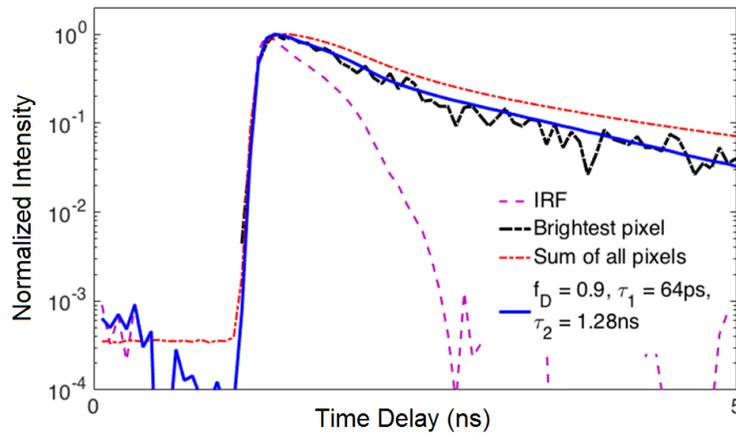
Fig. 4. Measured IRF, measured and fitted histograms.
