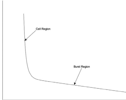
Fig. 1. Cell and burst regions. The  $P_L(N)$  plotted on the y-axis is on a log scale and the buffer size plotted on the x-axis is on a linear scale.
