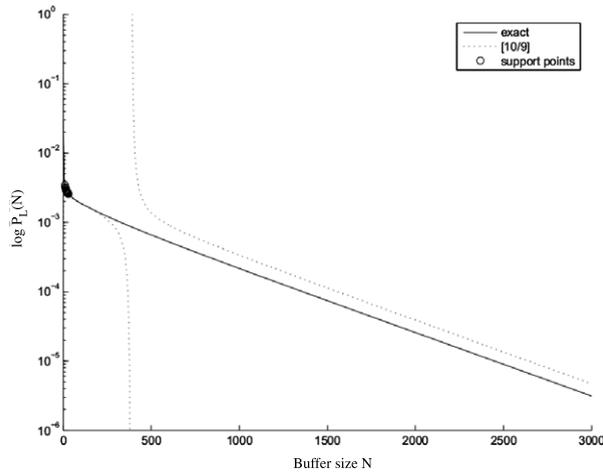
Fig. 2. Rational approximant for  $\log P_L(N)$  with a pole around  $N = 80$ .
