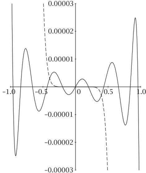
**Figure 6** Error plots of Chebyshev (solid line) and Taylor (dashed line) partial sums of degree 9 for  $\arctan(x)$ .
