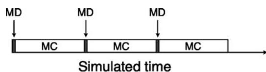
**Fig. 1** Schematic representation of the alternating MD/MC approach
