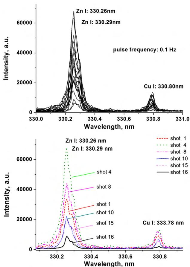
Fig. 2. Intensity fluctuation of successive dual-pulse LIBS spectra of brass measured at a laser pulse frequency of 0.1 Hz. (top figure) 20 individual spectra; (bottom figure) a choice of six spectra out of 20 shown in top figure.
