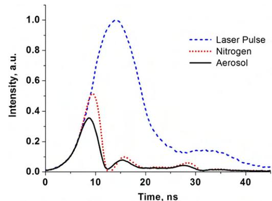
Fig. 7. Incident laser waveform (i.e., no breakdown) along with the transmitted laser waveforms recorded for pure nitrogen breakdown and for breakdown in the 75 nm mean diameter aerosol. Each waveform corresponds to the average of 100 shots, and all waveforms have the same intensity scale.
