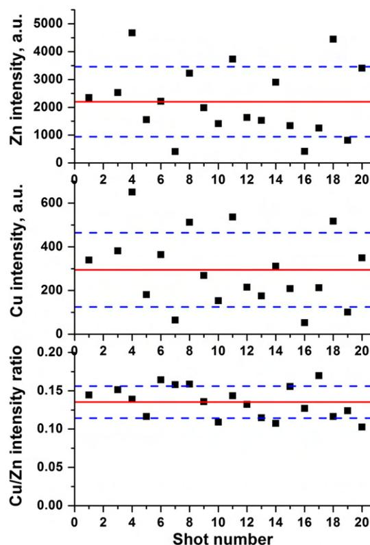
Fig. 3. The Zn and Cu line peak intensities of the 20 single spectra of Fig. 1 and their ratios. The full lines represent the average values while the dashed lines show the relative standard deviations: 57%, 58%, and 15% for Zn, Cu and the Cu/Zn ratio, respectively.
