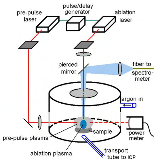
Fig. 1. Experimental arrangement for dual-pulse LIBS with orthogonal pre-pulse, absorption measurements of the pre-pulse energy, and ICP-OES.
