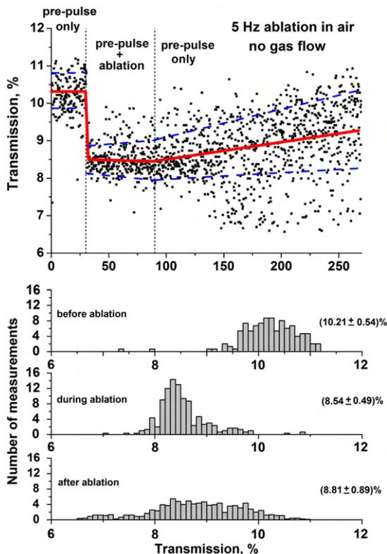
Fig. 6. (Top) transmission of the pre-pulse laser without and with mass ablation from the second laser in air without gas flow through the ablation cell. (bottom) evaluation of the transmission data before, during, and after ablation.
