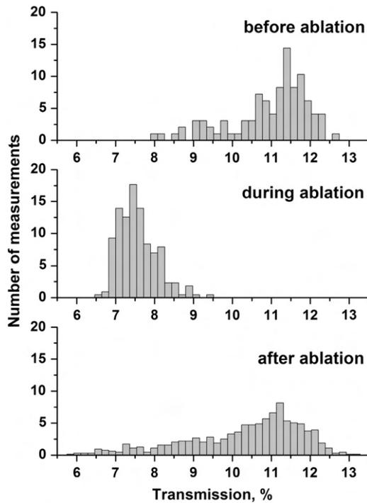
Fig. 5. Evaluation of the transmission measurements with 5 Hz laser pulse frequency displayed in the lower part of Fig. 5.
