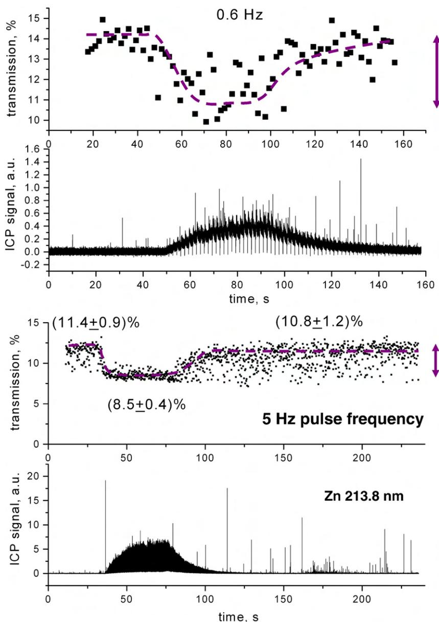
**Fig. 4.** The transmission of the pre-pulse laser without and with ablation of brass and the corresponding ICP-OES signal of the 213.8 nm Zn line in dependence on time. Ablation started at 45 s and 35 s and stopped at 95 s and 80 s at 0.6 and 5 Hz laser pulse frequency, respectively. The long ICP-OES signals represent the low particle washout of the ablation cell. The spikes in the ICP response are due to larger particles (see also [18]).
