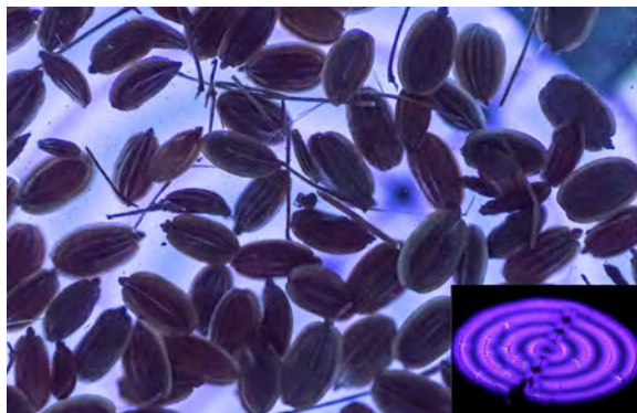
FIGURE 5 Example for food treatment by nonthermal atmospheric pressure plasma. Dill ( Anethum graveolens ) seeds treated with dielectric barrier discharge (DBD). Small photo: DBD with plasma turned on, ring-shaped electrode configuration. Taken from Ref. [85]. Reproduced with kind permission by the authors and Biblioteca Horticultura
