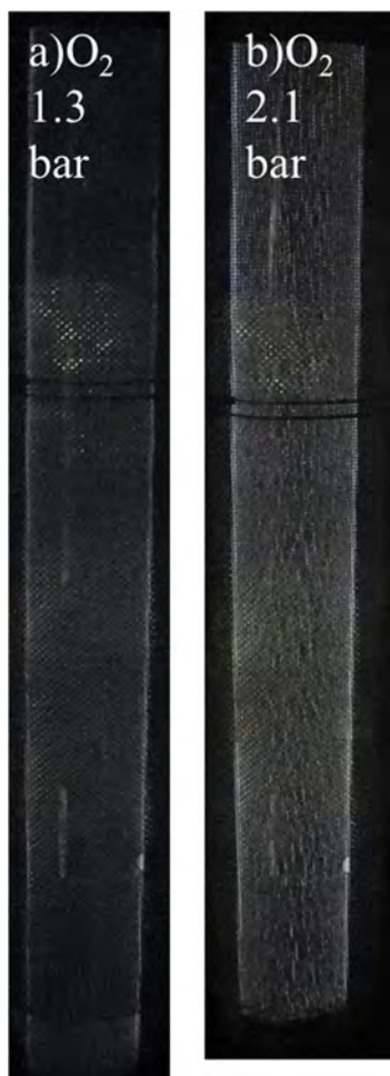
FIGURE 4 Images of 1 SLM O 2 DBD (exposure time 1/25 s) at (a) P = 1.3 bar, (b) P = 2.1 bar
