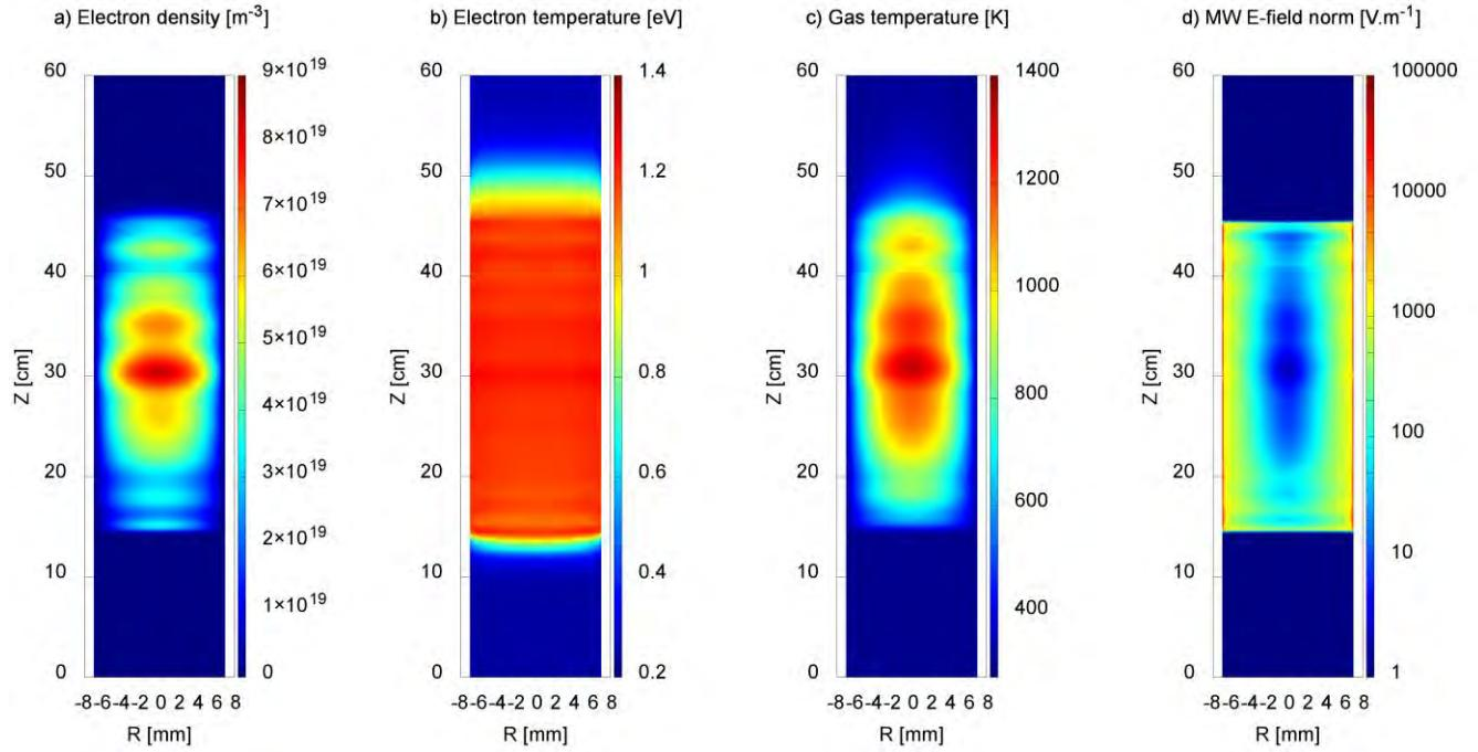
**Figure 2.** Electron density (a), electron temperature (b), gas temperature (c) and norm of the microwave electric field (d).
