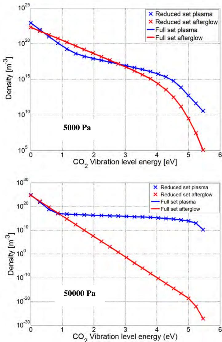
**Figure 4.** CO<sub>2</sub> vibrational distribution in the plasma (blue) and in the afterglow (red), using the full model (lines) and the reduced model (crosses).
