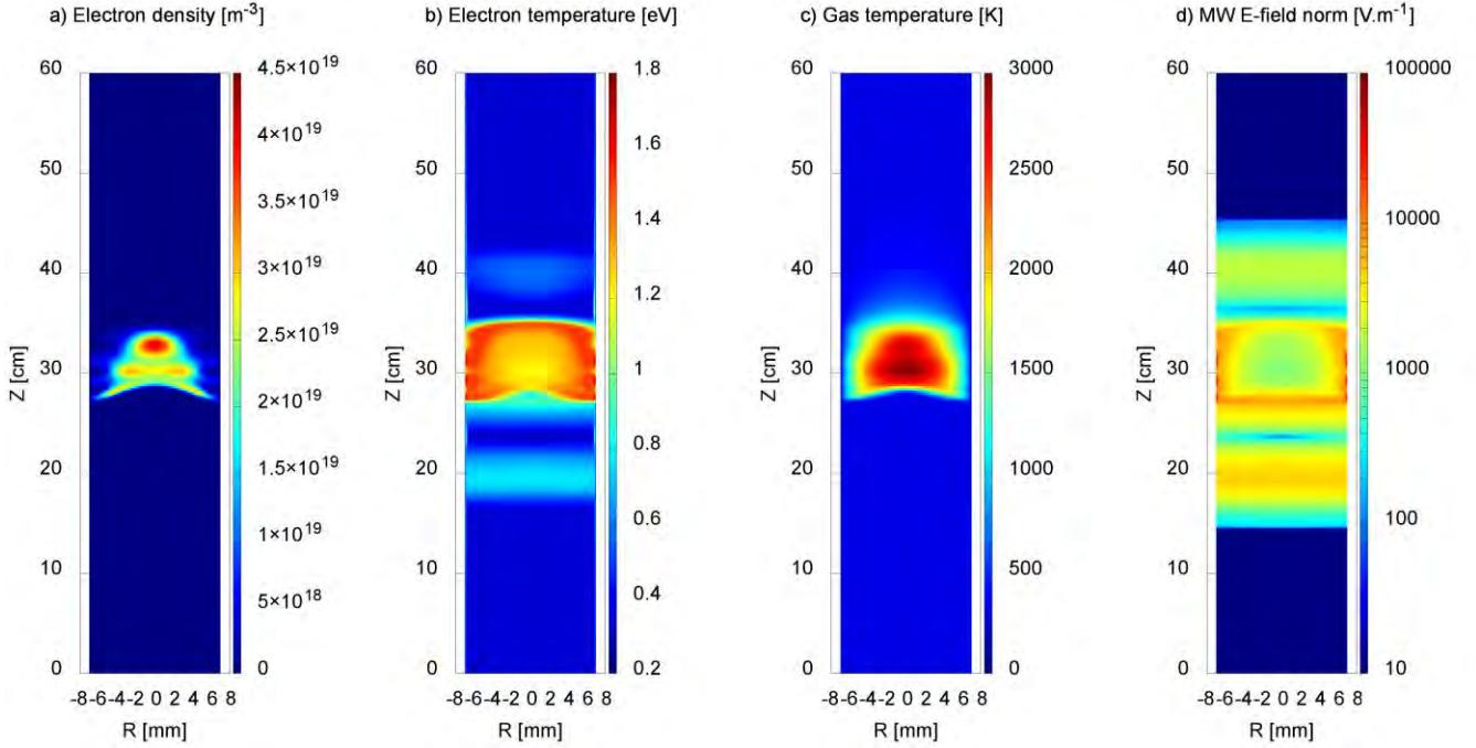
**Figure 3.** Electron density (a), electron temperature (b), gas temperature (c) and norm of the microwave electric field (d). Pressure:  $10^5$  Pa, Power: 100W, Gas flow: 500 sccm
