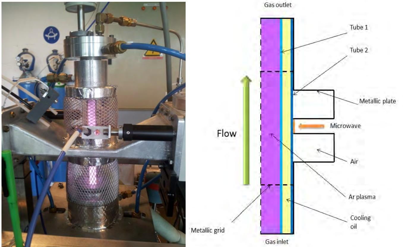
**Figure 1.** Microwave setup (on the left) and sketch of the computational domain (on the right)
