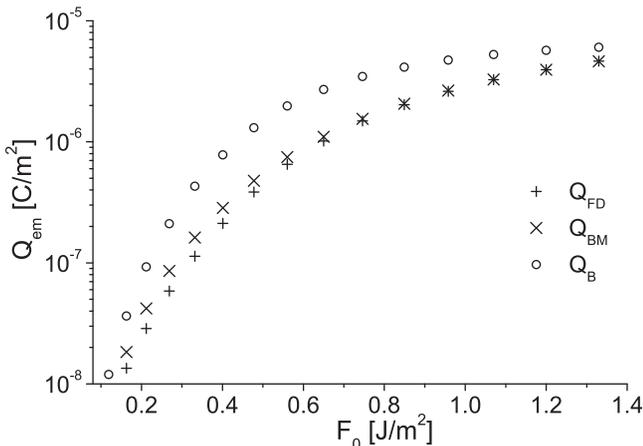
FIG. 6. The number of effectively emitted electrons as a function of the laser fluence, calculated by PIC-simulations assuming an electron flux calculated by the FD-theory, and a Maxwellian velocity distribution (FD), an electron emission flux taking into account the actual electron distribution and a Maxwellian velocity distribution (BM) and an electron emission flux as well as a velocity distribution based on the actual electron distribution (B).
