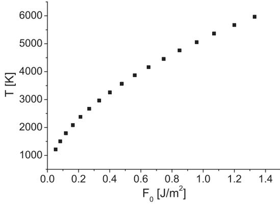
FIG. 3. The peak electron temperature corresponding to the energy distribution for simulations with different laser fluences.
