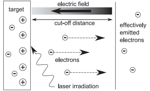
FIG. 1. A schematic representation of the model. The electrons in the target were modeled by the Boltzmann equation as well as by the FD-theory, the motion of emitted electrons in the computational area was modeled by the particle-in-cell code.
