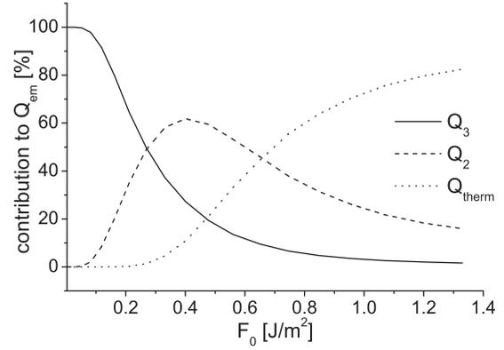
FIG. 4. The relative contributions of the 3PPE, 2PPE, and thermionic emission process, denoted by  $Q_3$ ,  $Q_2$ , and  $Q_{\text{therm}}$ , respectively, to the total emitted charge in percentages, as a function of the laser fluence.
