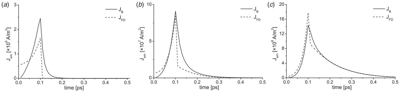
FIG. 5. The electron emission pulse shape resulting from the Boltzmann equation (solid) and calculated by the FD-theory (dashed) for laser fluences of 0.212, 0.478, and 0.849 J/m<sup>2</sup>.
