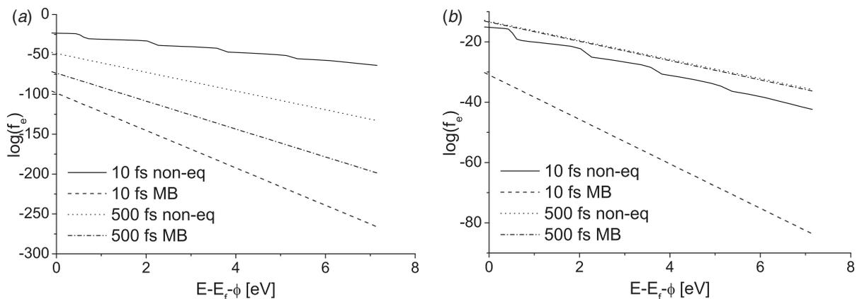
FIG. 2. The tails of the electron distributions for energies above the work function, during and after laser irradiation with a fluence of (a)  $F_0 = 0.05 \text{ J/m}^2$  and (b)  $F_0 = 0.85 \text{ J/m}^2$ . The labels non-eq and MB denote non-equilibrium distribution calculated by the Boltzmann equation, and a Maxwell tail of the Fermi distribution based on the corresponding internal energy and density, respectively.
