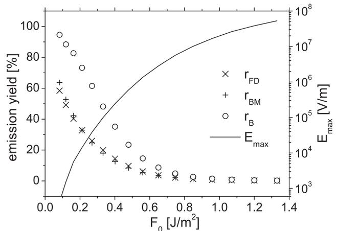
FIG. 7. The yield of effectively emitted electrons relative to the initially emitted charge  $Q_{init}$  as a function of the laser fluence, including the space charge effect for different laser fluences. The labels are as in Fig. 6. The solid curve shows the maximum value of the electric field above the target for each fluence.
