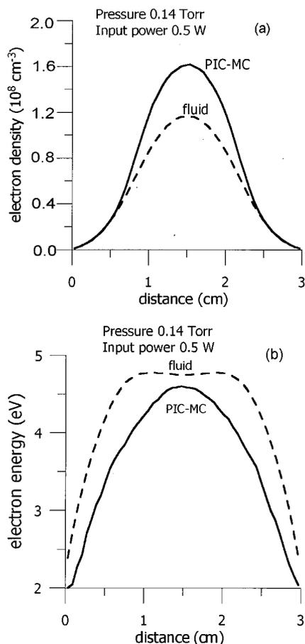
FIG. 4. Stationary state spatial distributions of: (a) the electron density and (b) the electron energy at a pressure of 0.14 Torr and an input power of 0.5 W, averaged over a rf cycle, calculated with the PIC–MC model (solid lines) and the fluid model (dashed lines).
