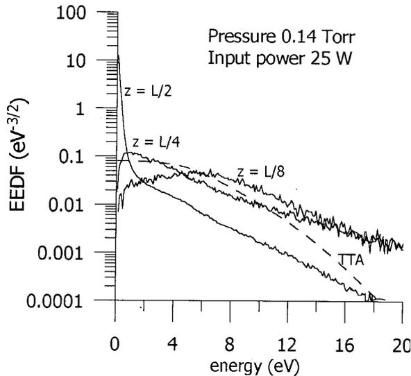
FIG. 3. EEDF at different distances between the electrodes at a pressure of 0.14 Torr and an input power of 25 W, calculated with the PIC-MC model (solid lines) and as a result of solving the homogeneous Boltzmann equation in the two-term approximation, used in the fluid model (dashed line) at an average electron energy of 5 eV.
