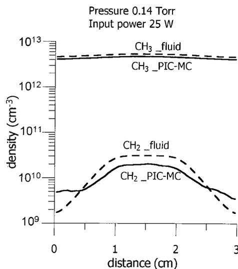
FIG. 6. Stationary state spatial distributions of CH<sub>2</sub> and CH<sub>3</sub> radicals at a pressure of 0.14 Torr and an input power of 25 W.
