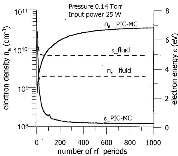
FIG. 1. Time dependence of the electron density  $n_e$  and the electron energy  $\epsilon$  averaged over a rf cycle in the center of the discharge at a pressure of 0.14 Torr and an input power of 25 W, calculated with the PIC–MC model (solid lines) and the fluid model (dashed lines).
