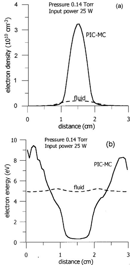
FIG. 2. Stationary state spatial distributions of: (a) the electron density and (b) the electron energy at a pressure of 0.14 Torr and an input power of 25 W, averaged over a rf cycle.
