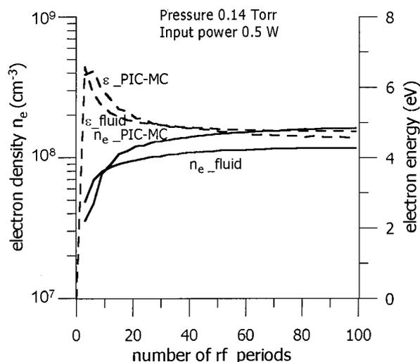
FIG. 5. Time dependence of the electron density  $n_e$  and the electron energy  $\epsilon$  averaged over a rf cycle in the center of the discharge at a pressure of 0.14 Torr and an input power of 0.5 W, calculated with the PIC–MC model (solid lines) and the fluid model (dashed lines).
