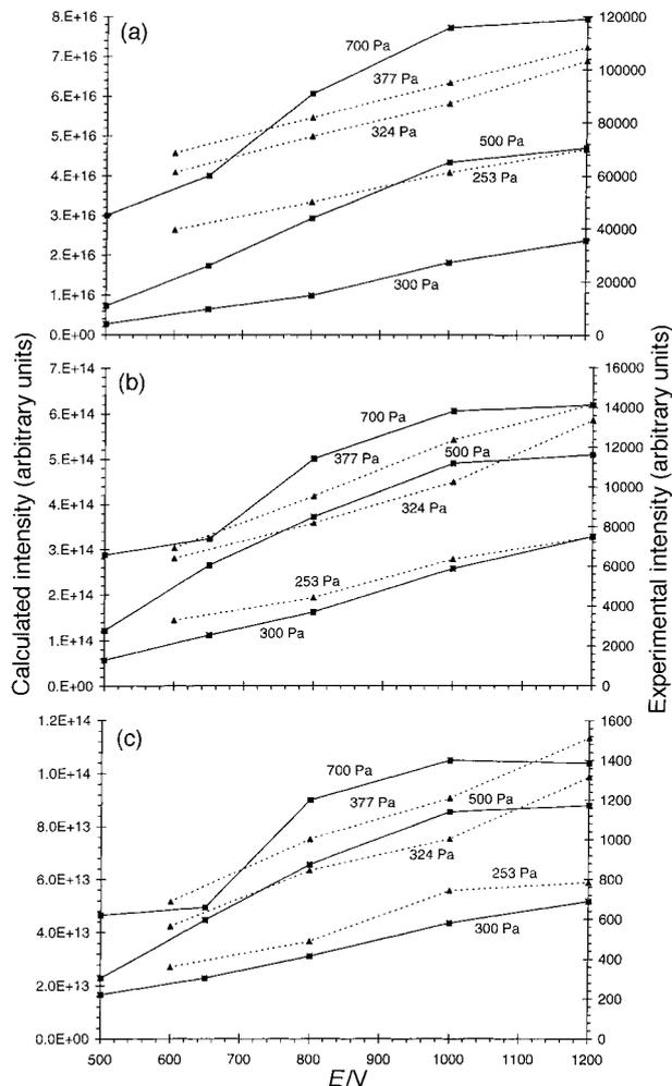
**Fig. 6** Calculated spectral line intensities of some argon atom lines in a Grimm-type glow discharge cell, integrated over the entire cell axis, as a function of voltage for three pressures (solid lines, left axis), and comparison with experimental data<sup>28</sup> (dashed lines, right axis). (a)  $\lambda = 750.39$  nm (originating from a 4p level); (b)  $\lambda = 427.22$  nm (originating from a 5p level); and (c)  $\lambda = 592.88$  nm (originating from a 7s level).
