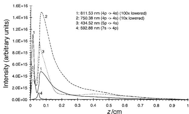
**Fig. 4** Calculated spectral line intensities of some argon atom lines in a Grimm-type glow discharge cell at the cell axis, as a function of distance from the cathode (at 800 V, 500 Pa, 28 mA).
