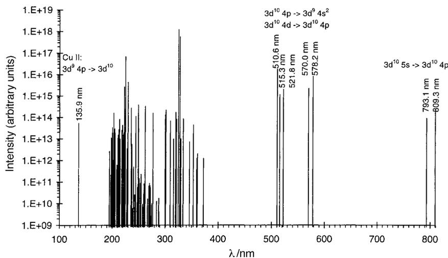
**Fig. 2** Calculated spectrum of the copper atom and ion lines in a Grimm-type glow discharge cell, integrated over the entire cell axis, to simulate end-on observation (at 800 V, 500 Pa, 28 mA).
