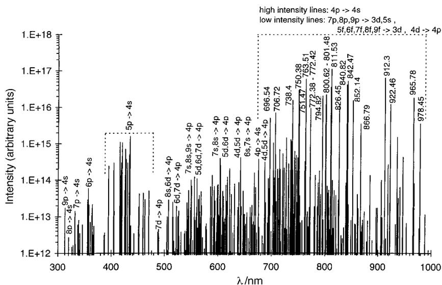
Fig. 1 Calculated spectrum of the argon atom lines in a Grimm-type glow discharge cell, integrated over the entire cell axis, to simulate end-on observation (at 800 V, 500 Pa, 28 mA).
