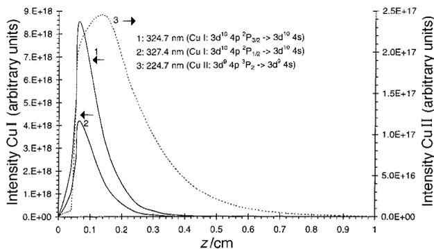
**Fig. 5** Calculated spectral line intensities of some copper atom and ion lines in a Grimm-type glow discharge cell at the cell axis, as a function of distance from the cathode (at 800 V, 500 Pa, 28 mA).
