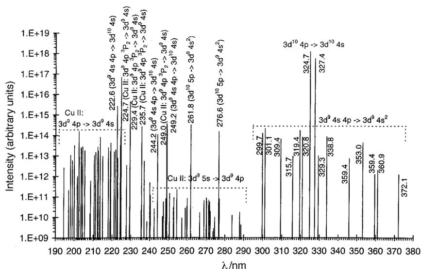
**Fig. 3** Calculated spectrum of the copper atom and ion lines in a Grimm-type glow discharge cell, integrated over the entire cell axis, to simulate end-on observation (at 800 V, 500 Pa, 28 mA): detail of the 200–400 nm range.
