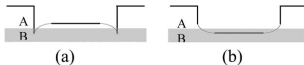
Fig. 4 Sketch of typical crater profiles: (a) with convex crater edge, (b) with concave crater edge.
