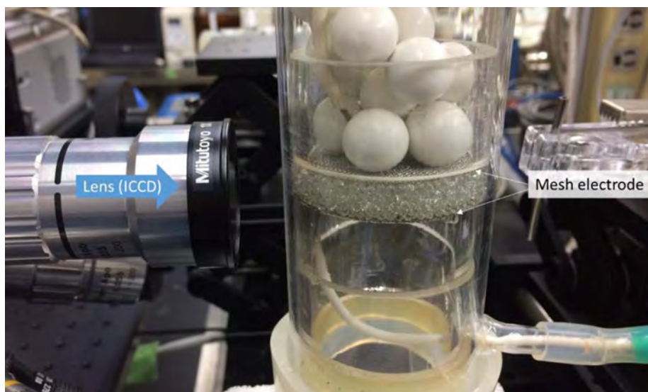
Fig. 2. Experimental configuration of the packed bed plasma reactor, used for ICCD imaging.
