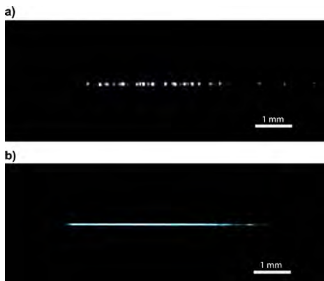
FIG. 12. Optical breakdown patterns from a horizontal laser beam (a) in degassed NaCl solution, with a low number density of nanobubbles, and (b) in the same solution after 24 h exposure to the open atmosphere, where the density has increased, as easily deduced from the continuous and brighter emitted light. Reprinted with permission from N. F. Bunkin et al. , J. Phys. Chem. B 120 (7), 1291–1303 (2016). Copyright 2016 American Chemical Society.
