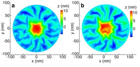
Height of the initial buckled graphene state with the bias voltage set to 3 V and the central temperature set to 300 K.
