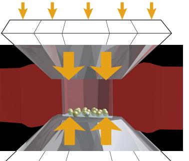
Our pressure gauge consists of nanoshells, nanoparticles with a silicon core and metallic shell. Their optical response can be engineered to be situated in a part of the spectrum where no other effects occure. Also, nanoshells give a stronger signal since they rely on extinction and not fluorescence. Furthermore, due to their smaller size compared to the rubies they provide the posibility of generating a pressure map of
