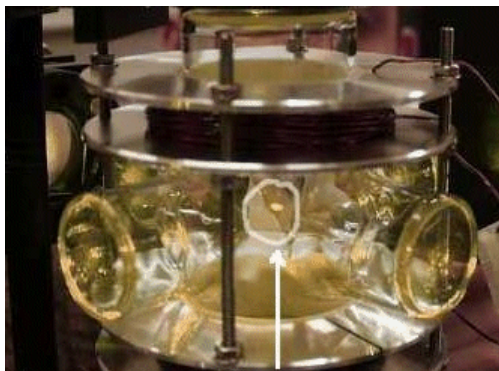
Figure 1.5: A magneto-optical trap with a cloud of trapped atoms (indicated by the arrow). The glass cell is vacuum-pumped, and has protrusions where the cooling laser beams enter. A coil for the magnetic quadrupole trapping is also visible on top and at the bottom of the cell.
