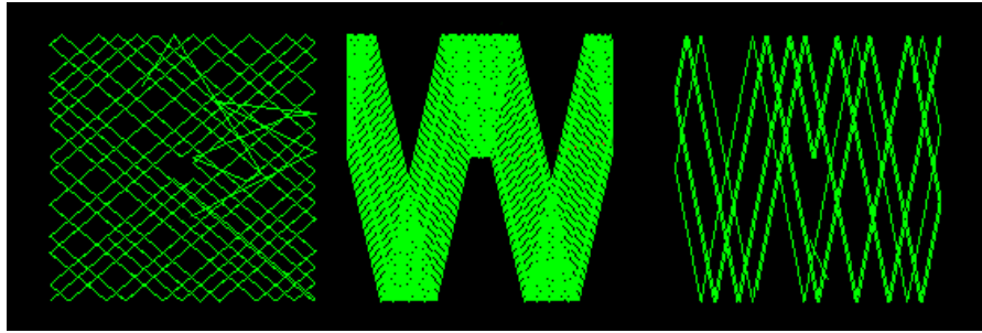
Figure 5.15: When the faces of the scintillator are perfectly polished, the photon often describes geometric trajectories. Some patterns are shown, with a perpendicular view to the scintillator face.
