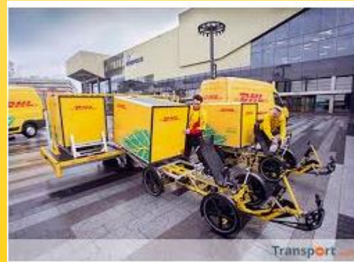
Electric bikes with replaceable containers require two couriers versus one courier in a van.
