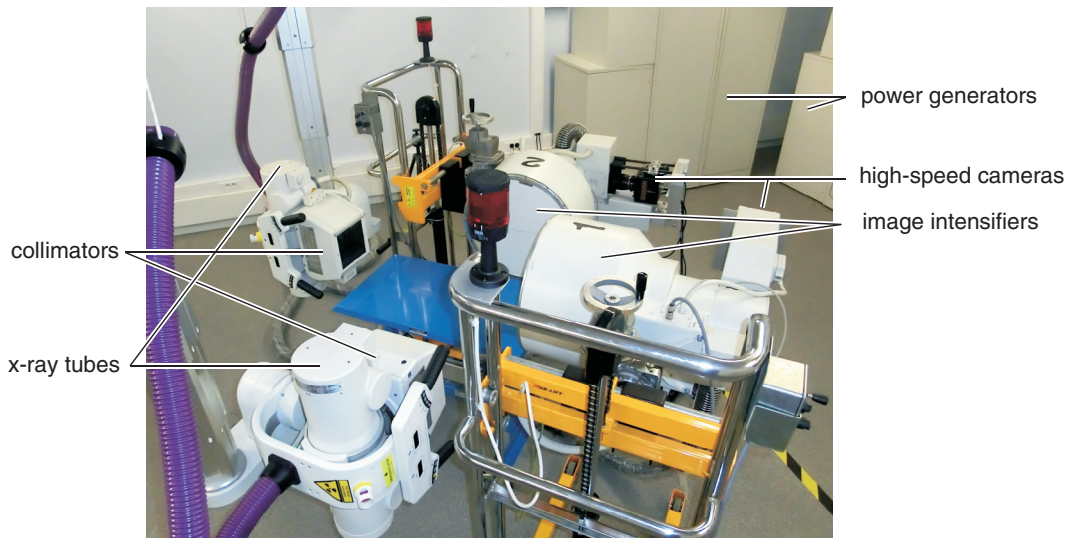
Figure 1. Biplanar x-ray video set-up at the University of Antwerp. Note that the x-ray sources (tubes) and beam collimators are attached to ceiling rails, while the image intensifiers and attached cameras are mounted on trolleys. The four main units (two sources and two detectors) are height adjustable and tiltable to allow for different beam orientations.
