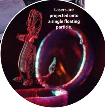
Lasers are projected onto a single floating particle.
