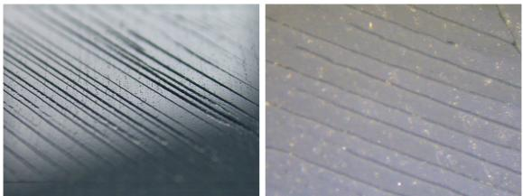
Close-up photos showing the tiny pits caused by the salt crystals. Try zooming in for a better view. Left picture taken using the camera macro-function, right picture taken through a microscope at 10x magnification: here the white salt stuck in the pits is still visible. For reference: nozzle diameter of our 3D-printers is 0.4mm, so the extrusion lines are about 0.4mm apart also.
