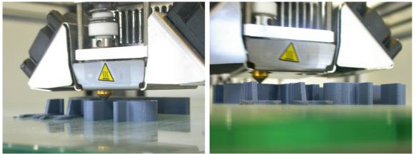
Printing several custom cable clamps in one batch. They show no sign of lifting corners whatsoever. Note that the salt is well visible at this low angle of view, giving a dusty appearance to the glass.
