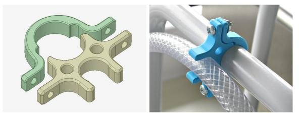
Clamps like these can be printed well too. This one was particularly difficult to print using other bonding methods, due to its small base area and its big chamfers that exerted a lot of warping force, and its 100% infill for mechanical strength. On a bare glass plate, I could not print it at all. When using the glue stick method, I had to retry a few times because it still warped and came off. Not so with the salt method.
