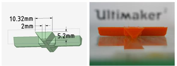
The only items of which corners did lift severely, were these specially designed "warptests": inverted prisms with a very small base (2mm), a very wide top (10mm), and big chamfered corners, which exert a lot of warping stress and tend to pry off the model. It is printed with 100% fill-in, for maximum shrinking- and
