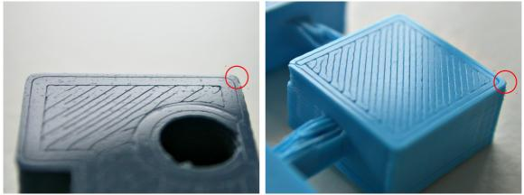
The typical (not) lifting of corners, on typical 3D-models: in a corner, an edge of 0.3mm wide might lift a little bit. That is usually all. See the right corners in both models (although hardly visible, try zooming in). For reference: the round hole in the left photo is 4.5mm diameter. The brick on the right photo is 10mm x 10mm x 5mm. Both are 100% filled. Also notice the tiny pits created by the salt in both samples, which look similar to corrosion-pits in metals.
