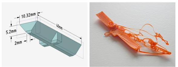
This inverted prism could not be printed anymore: it came off halfway and produced some nice spaghetti before I aborted the print. Corners curled up too much (clearly visible in front), and then the print head hit them hard and knocked the model off the plate. So this model would need brims or a raft to print successfully. This warptest shows the limitations of the salt method: no upside-down prisms or pyramids.
