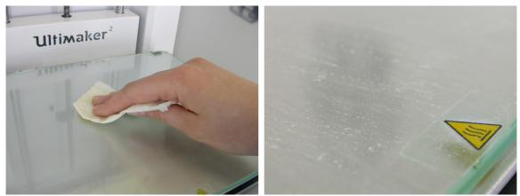
Keep wiping the glass plate very gently and lightly: first from left to right, then from back to front until the water evaporates. This leaves an even, thin mist of salt stuck to the plate. On the close-up photo, contrast is artificially enhanced in Photoshop, otherwise the salt would be very hard to see. In reality the glass plate just looks somewhat matt and dusty.
