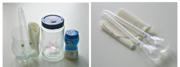
This is all you need for "the salt method": paper tissue, glass jar, salt, tap water, and two cheap pipettes: one for salt water and one for pure tap water. I labeled my pipettes with  $H_2O$  for the pure tap water and NaCl for the salt water so I can easily recognise them.
