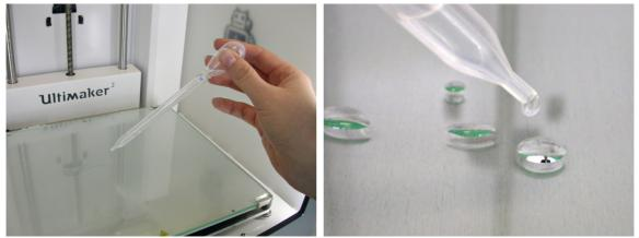
Applying a few drops of salt water: these drops usually stay quite round, and tend to regroup, instead of spreading out into a thin layer. This is a good sign. Instead of applying the drops directly to the glass plate, it is safer to apply them to a paper tissue first, and then use the moist tissue to wipe the glass plate. That reduces the risk of spilling water into the printer electronics.
