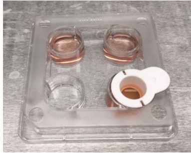
Fig. 2 PAFs are placed in a mini cell strainer immersed in cryoprotective agents (ES and VS) in a 4-well plate. Mini cell strainers are transferred with tweezers between different media and equally serve as cryo-container when they are plunged in LN 2
