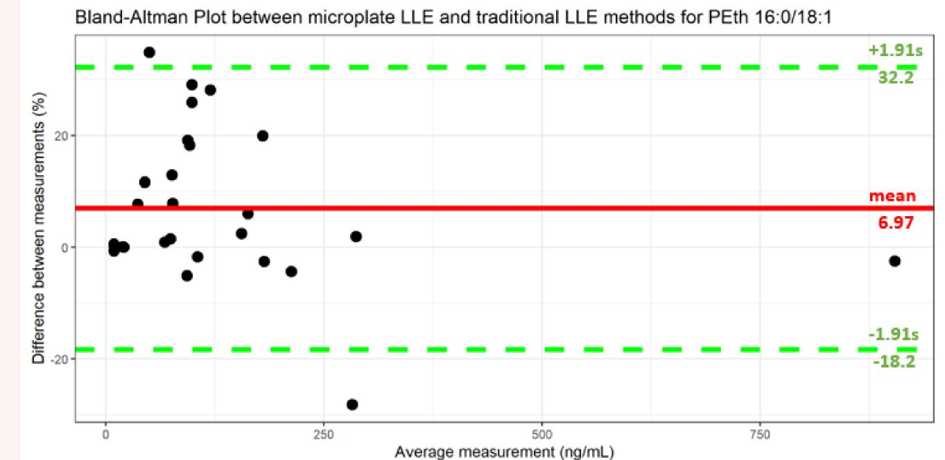
The microplate liquid-liquid extraction (LLE) method was compared with the previously validated traditional LLE approach using authentical samples. Our findings demonstrate an agreement between the two methods, confirming that microplate LLE is a reliable and efficient alternative for routine analysis. These results highlight the potential of microplate LLE as a successful technique in routine laboratories.
