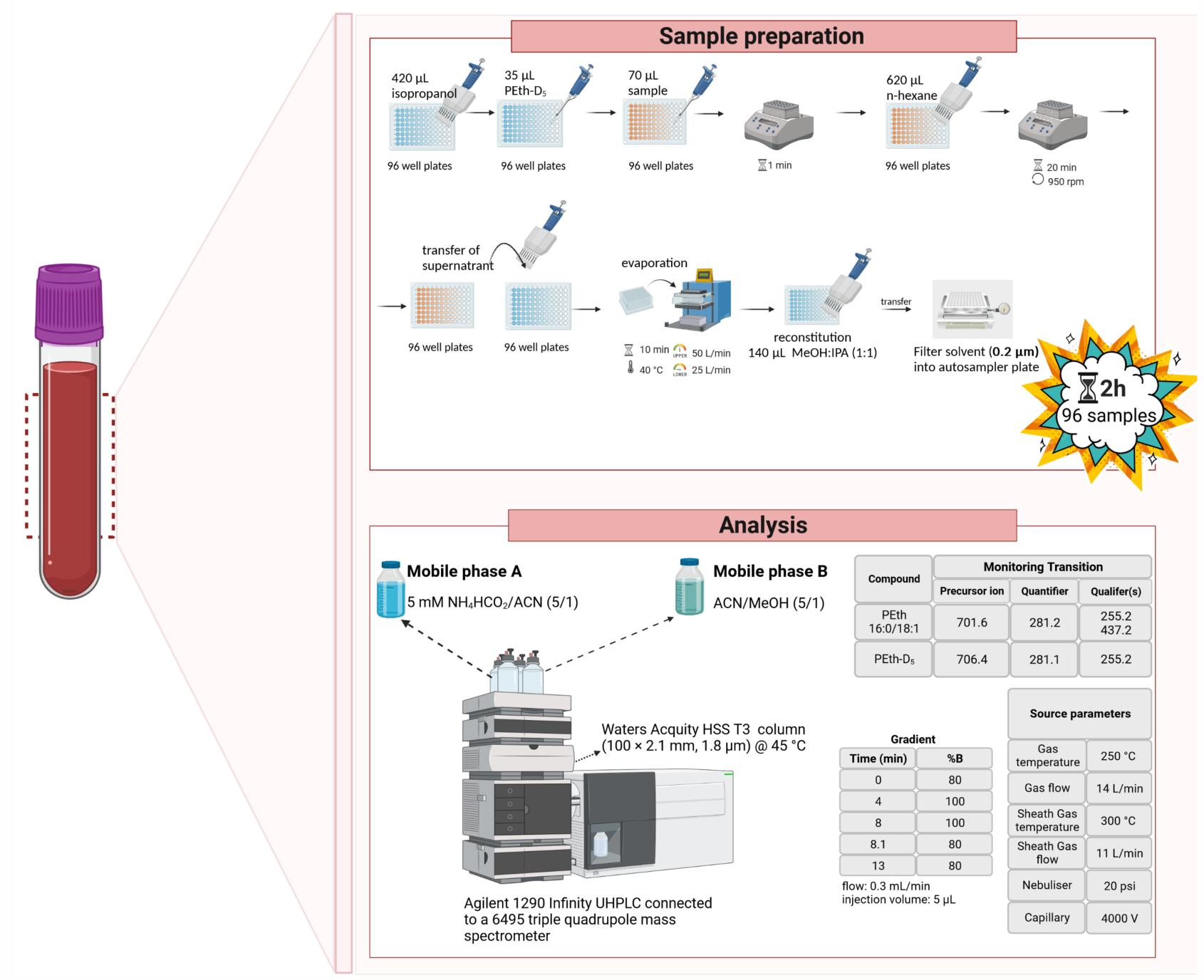
The current methodology is based on previously published method. ¹ The old method uses 30% more sample volume (100 µl), and 30% more solvents volumes (50 μl IS; 600 μl isopropanol; 900 μl hexane; 200 μl reconstitution solvent). Due to the 96 well plates, the multi-pipette, and the evaporation system, the sample preparation of 96 samples would take 50% less time. Therefore, this new method saves time, sample and solvent volumes when analysing a large amount of samples.
