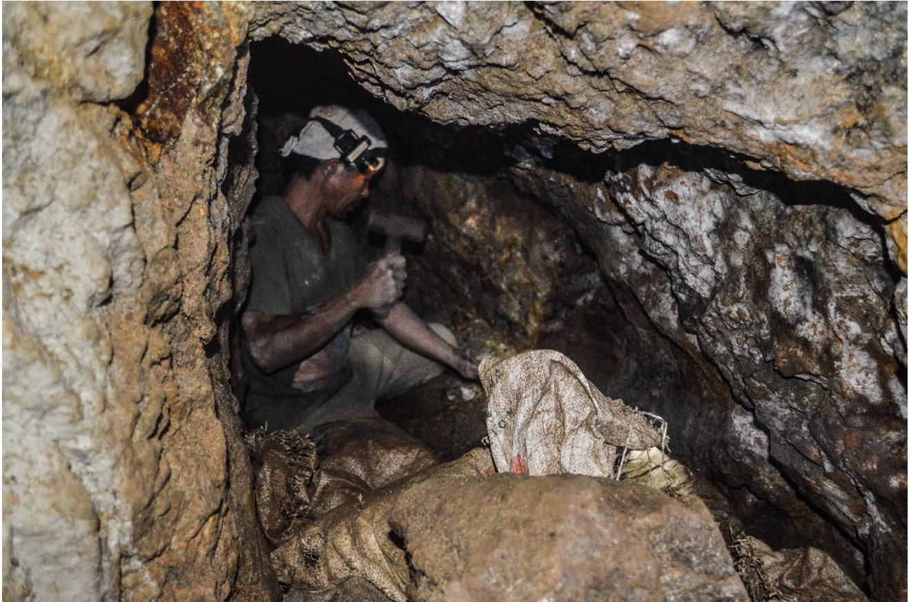
Figure 19. Chisel and hammer are among the most frequently mentioned tools by workers in this survey. In this image, a miner makes use of both tools while accumulating sacks of ore in the narrowness of the tunnel
