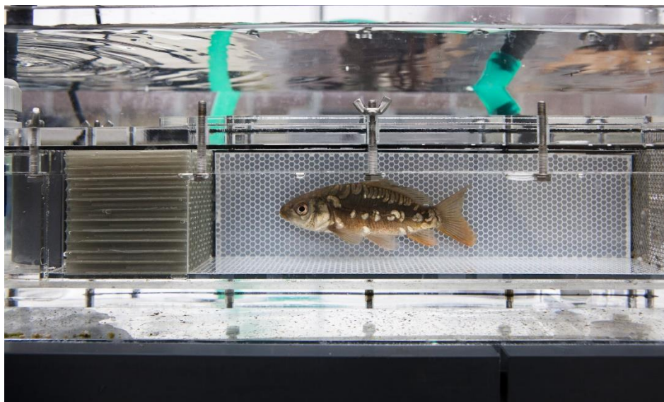
A juvenile common carp swimming in a respirometer raceway at the ECOSPHERE lab.
