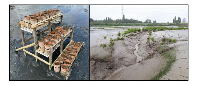
Picture on the left: A marsh organ, a device placed in tidal marshes to measure the effects of inundation time. Picture on the right: An example of an intertidal mudflat (Lillo-Potpolder, located along Scheldt estuary), showing pioneer species (Vaucheria algae and Aster tripolium) colonizing along the fringes of a tidal channel.
