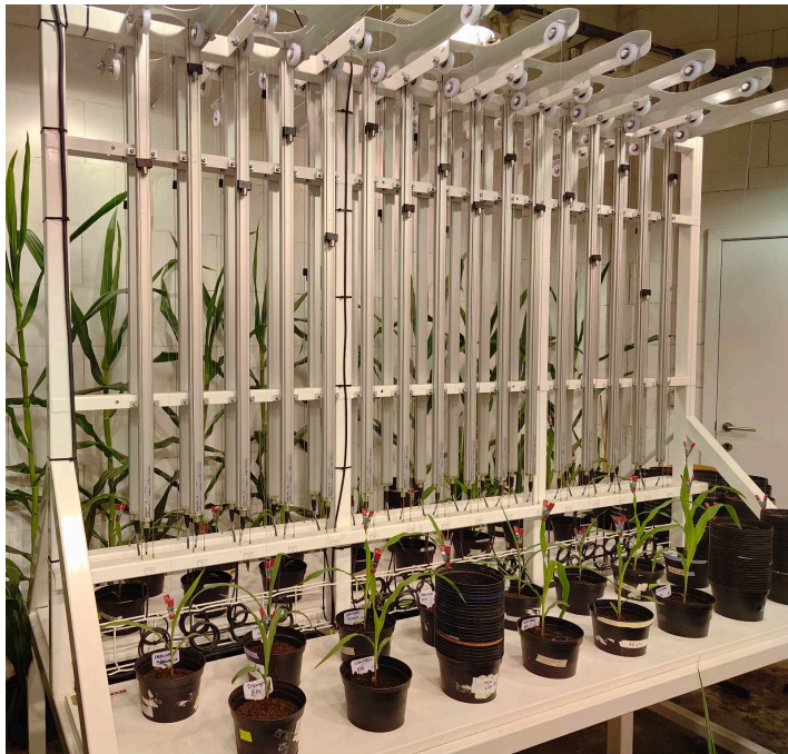
Study of dynamic changes using the LLT, e.g., yellow-marked timepoints indicate re-watering of drought-stressed plants; increase in leaf elongation rate (LER) occurs almost instantaneously
