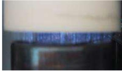
Figure 11 : Picture of a filamentary discharge in a DBD [73].
