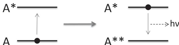
Figure 22 : Principle of the photon emission.
