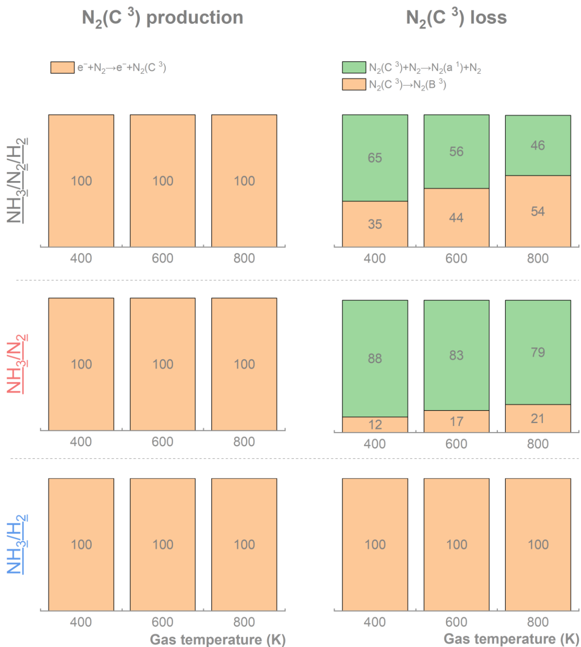
Figure S20. Contribution of main elementary reactions to the production (left plots) and loss (right plots) of N_2(C^3) in a 1 v/v% NH_3 mixture with different balance gases: a 1:3 molar ratio of N_2/H_2 (top row), N_2 (middle row), and H_2 (bottom row). Within each plot, results are shown from left to right for three gas temperatures, T_g = 400, 600, and 800 K. The specific energy input is 1.2 \text{ J/cm}^3 , corresponding to 20 \text{ W} at a total flow rate of 1 \text{ SLPM} . The E/N values used for the analysis are listed in Table S12.
