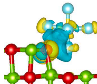
Fig. 7. Differential charge distribution of SF 6 over the step-shape MgO (001) surface. The yellow region indicates an increase in charge density and the cyan region indicates a decrease.
