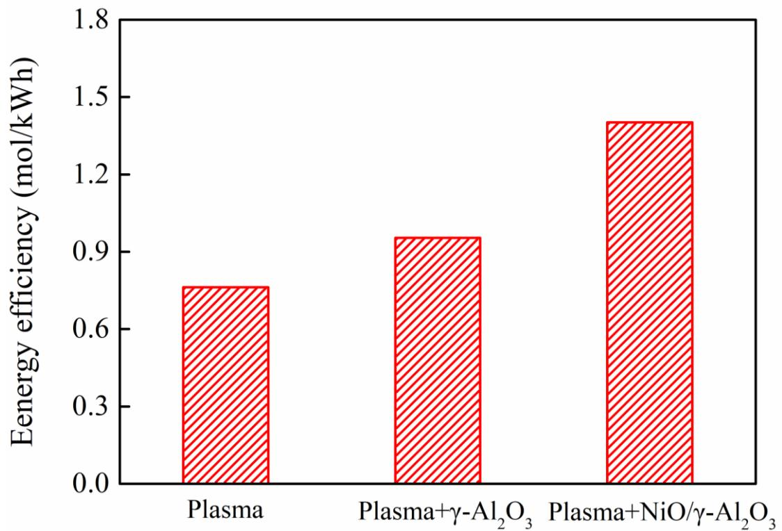
**Figure S12.** Energy efficiency in the case of plasma, plasma +  $\gamma$ -Al<sub>2</sub>O<sub>3</sub> and plasma + NiO/ $\gamma$ -Al<sub>2</sub>O<sub>3</sub>
