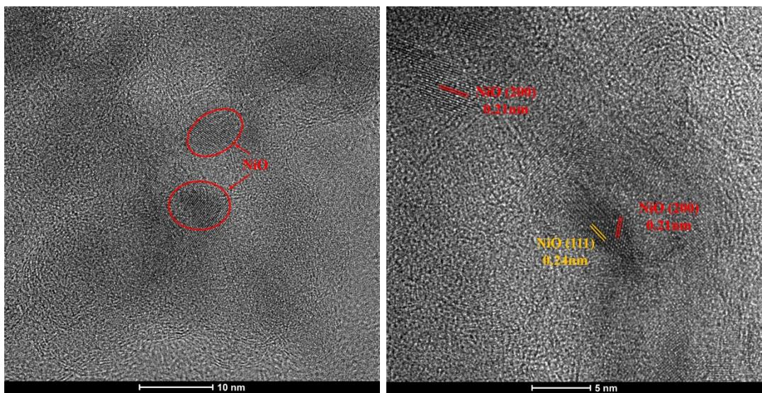
**Figure S17.** HRTEM results of the 10 wt.% NiO/γAl<sub>2</sub>O<sub>3</sub> catalysts.
