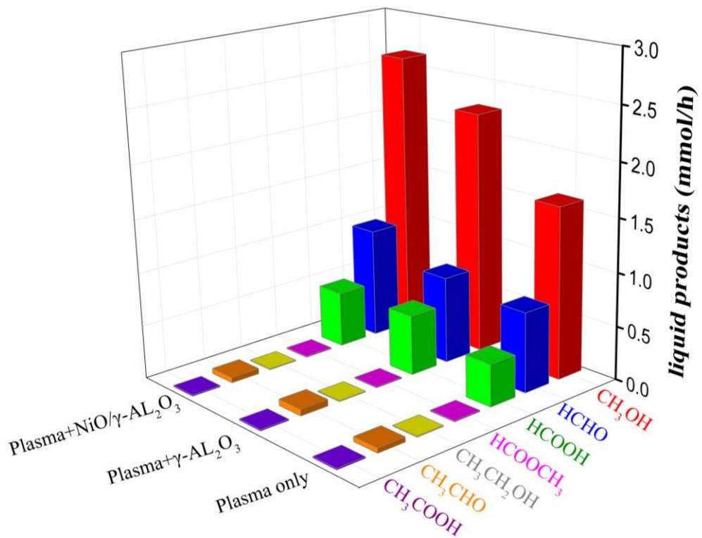
**Figure S7.** Liquid products distribution after 2-hour  $\text{CH}_4/\text{O}_2$  NTP operation, for plasma only, plasma +  $\gamma\text{-Al}_2\text{O}_3$  beads and plasma +  $\text{NiO}/\gamma\text{-Al}_2\text{O}_3$  catalyst.
