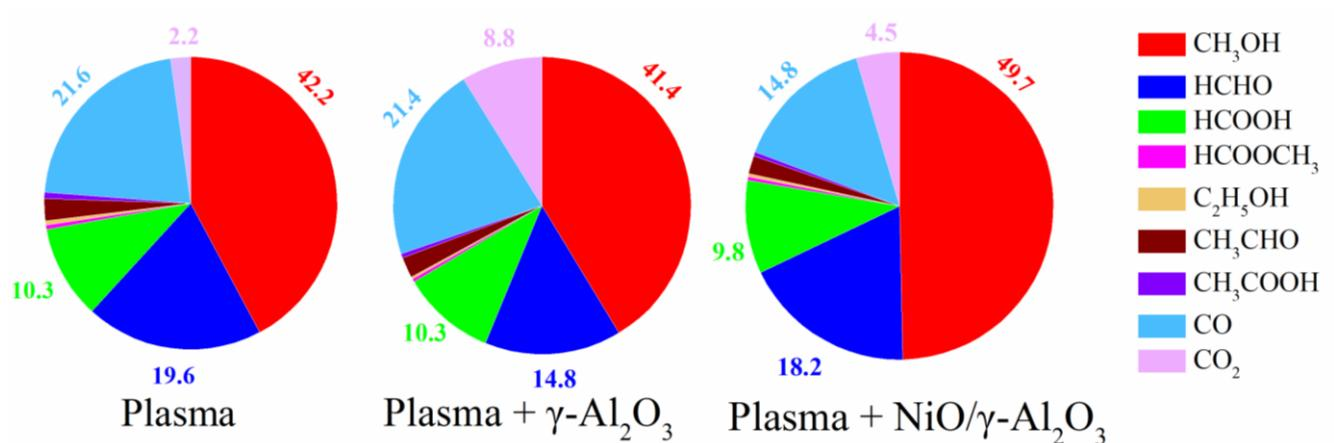
**Figure S8.** Products selectivity distribution of SOMTM (Carbon based), for all gas and liquid products, in the case of only plasma, plasma with  $\gamma\text{-Al}_2\text{O}_3$  beads, and plasma with (10 wt%)  $\text{NiO}/\gamma\text{-Al}_2\text{O}_3$  catalyst
