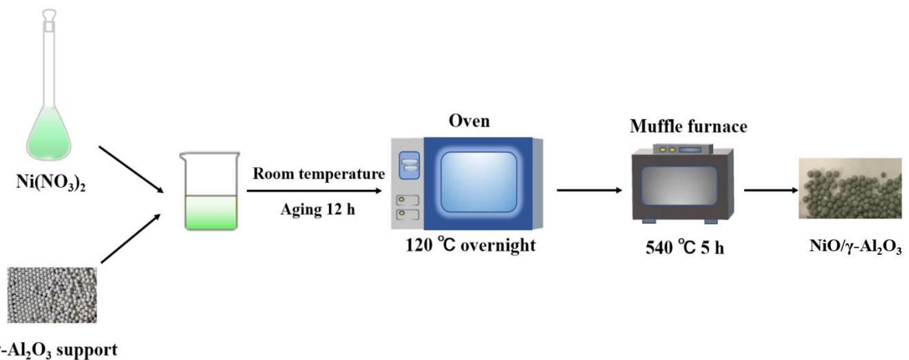
**Scheme S1.** Schematic diagram of the Ni catalyst preparation procedure
