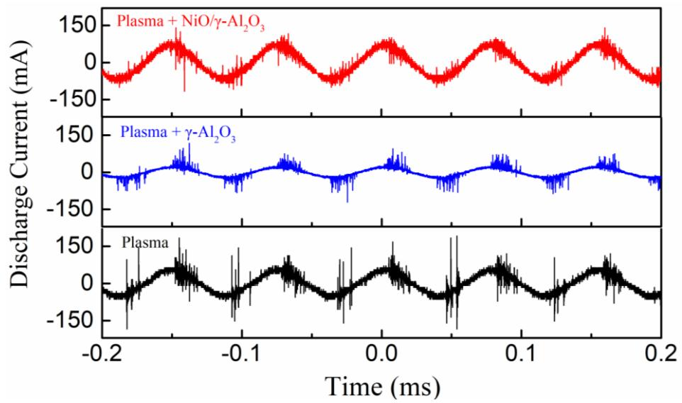
**Figure S11.** Discharge current in the case of plasma, plasma+ $\gamma$ -Al<sub>2</sub>O<sub>3</sub>, and plasma + NiO/ $\gamma$ -Al<sub>2</sub>O<sub>3</sub>
