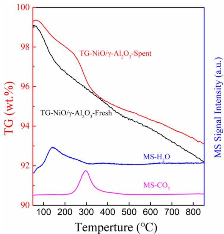
**Figure S21.** TG-MS of the fresh (black color) and spent (red color) NiO/γ-Al<sub>2</sub>O<sub>3</sub> catalyst (fresh catalyst was used as a contrast)
