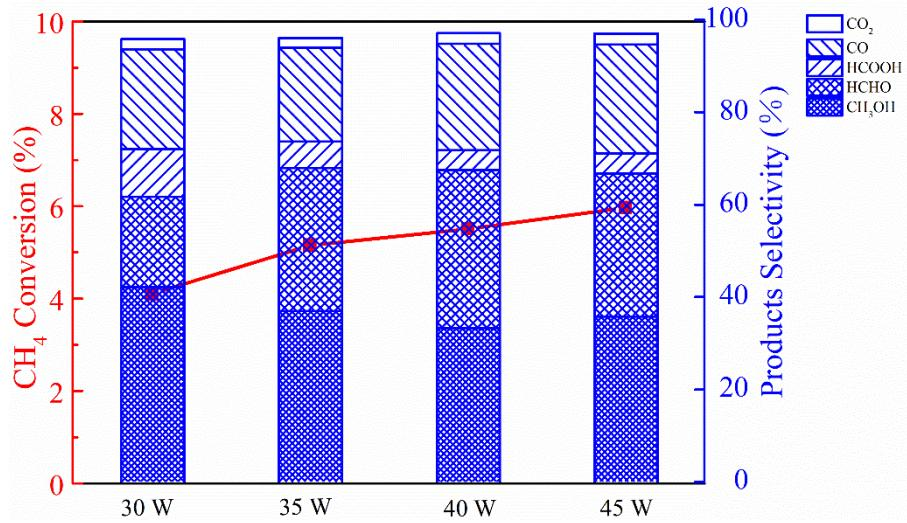
**Figure S5.** The influence of discharge power on  $\text{CH}_4$  conversion and product selectivity
