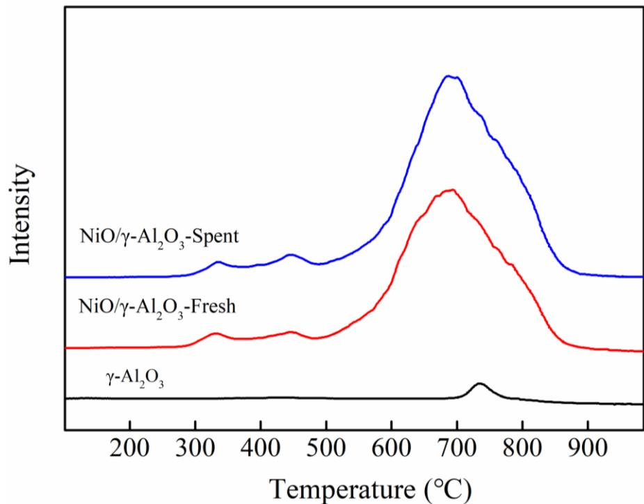
**Figure S23.** TPR profile of the fresh and spent NiO/γ-Al<sub>2</sub>O<sub>3</sub> catalyst
