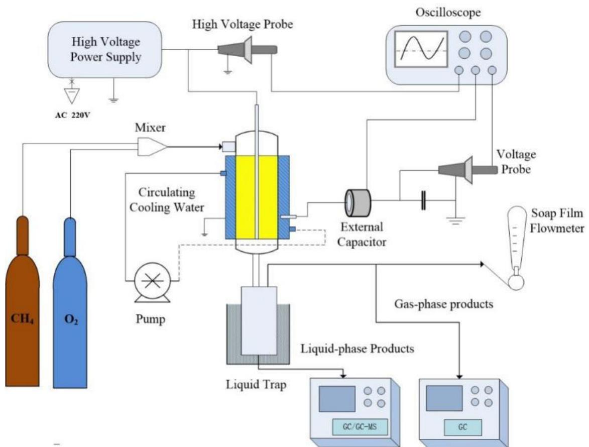
**Scheme S2.** Schematic diagram of the experimental setup for plasma catalytic SOMTM by molecular oxygen
