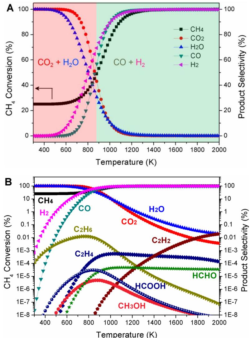
**Figure S1.** (A) Thermodynamic equilibrium of CH<sub>4</sub> conversion upon oxidation by O<sub>2</sub> (left axis), and product selectivity (right axis), as a function of reaction temperature at atmospheric pressure (mole ratio: CH<sub>4</sub>/O<sub>2</sub> = 2/1). (B) Product selectivity in logarithmic scale, illustrating the products with lower thermodynamic equilibrium selectivity, including CH<sub>3</sub>OH.
