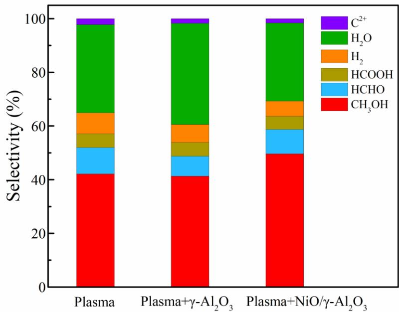
**Figure S9.** Products selectivity of SOMTM (hydrogen based) using only plasma, plasma with  $\gamma$ -Al<sub>2</sub>O<sub>3</sub> beads, and plasma with (10 wt.%) NiO/ $\gamma$ -Al<sub>2</sub>O<sub>3</sub> catalyst (400 ml/min CH<sub>4</sub>, 200 ml/min O<sub>2</sub>, 85°C circulating water, 1.25g NiO/ $\gamma$ -Al<sub>2</sub>O<sub>3</sub> catalyst, 30W discharge power and 0.375 s residence time).
