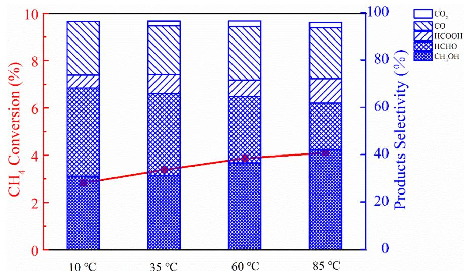
**Figure S4.** The influence of grounding electrode temperature on  $\text{CH}_4$  conversion and product selectivity in  $\text{CH}_4/\text{O}_2$  plasma
