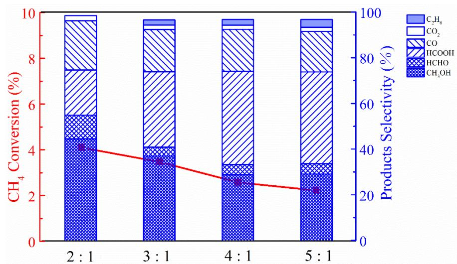
**Figure S3.** The influence of different  $\text{CH}_4/\text{O}_2$  molar ratio on  $\text{CH}_4$  conversion and product selectivity
