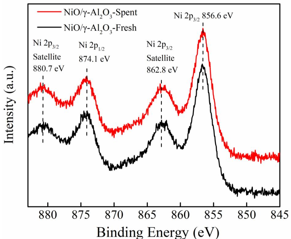
**Figure S24.** XPS profile of the fresh and spent NiO/γ-Al<sub>2</sub>O<sub>3</sub> catalysts
