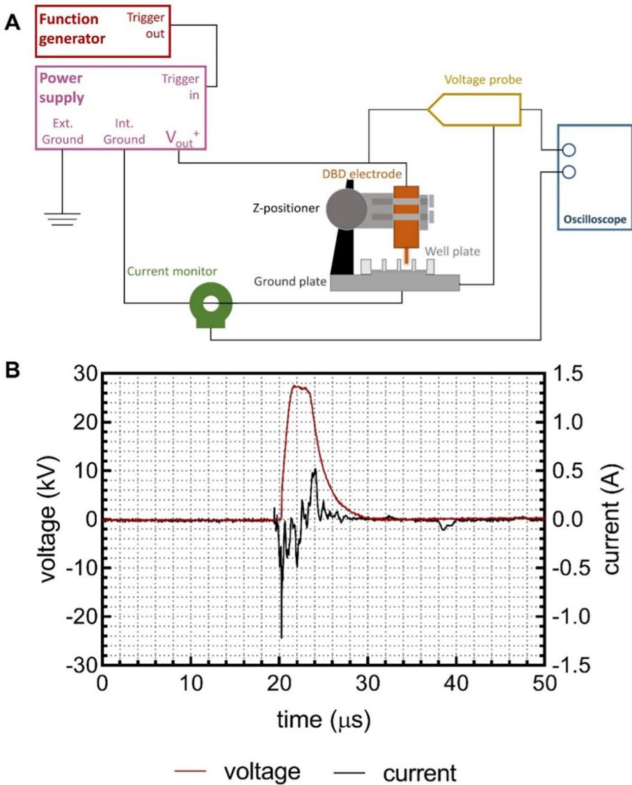
**Fig. 3** Experimental setup for power measurements. **(A)** Schematic of the experimental setup, where the voltage and current of the DBD plasma discharge were measured using a voltage probe and current monitor, respectively, and recorded on an oscilloscope. **(B)** Sample voltage and current waveform
