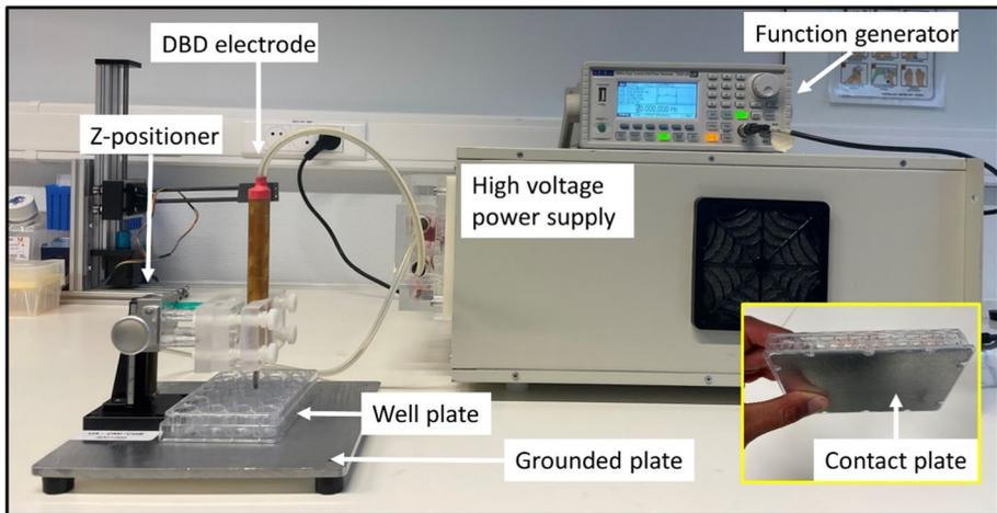
**Fig. 1** The microsecond-pulsed DBD plasma system used in this study. This system was also used in our previous plasma medicine work [27, 34, 35]. A contact plate (yellow insert) was used to fit within the well plate frame to ensure that the bottom of the well was in direct contact with the grounded plate (Color figure online)
