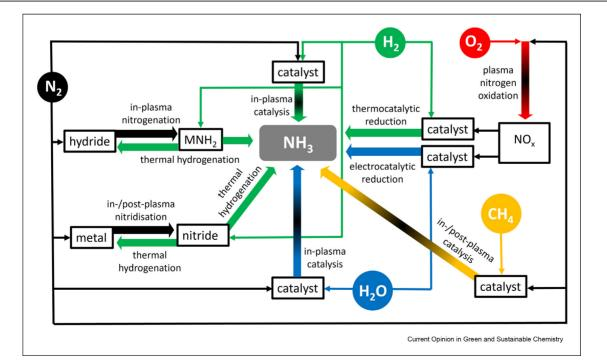
Various plasma-based pathways of nitrogen fixation into NH<sub>3</sub> include direct plasma catalysis, plasma with subsequent catalysis, and chemical looping.
