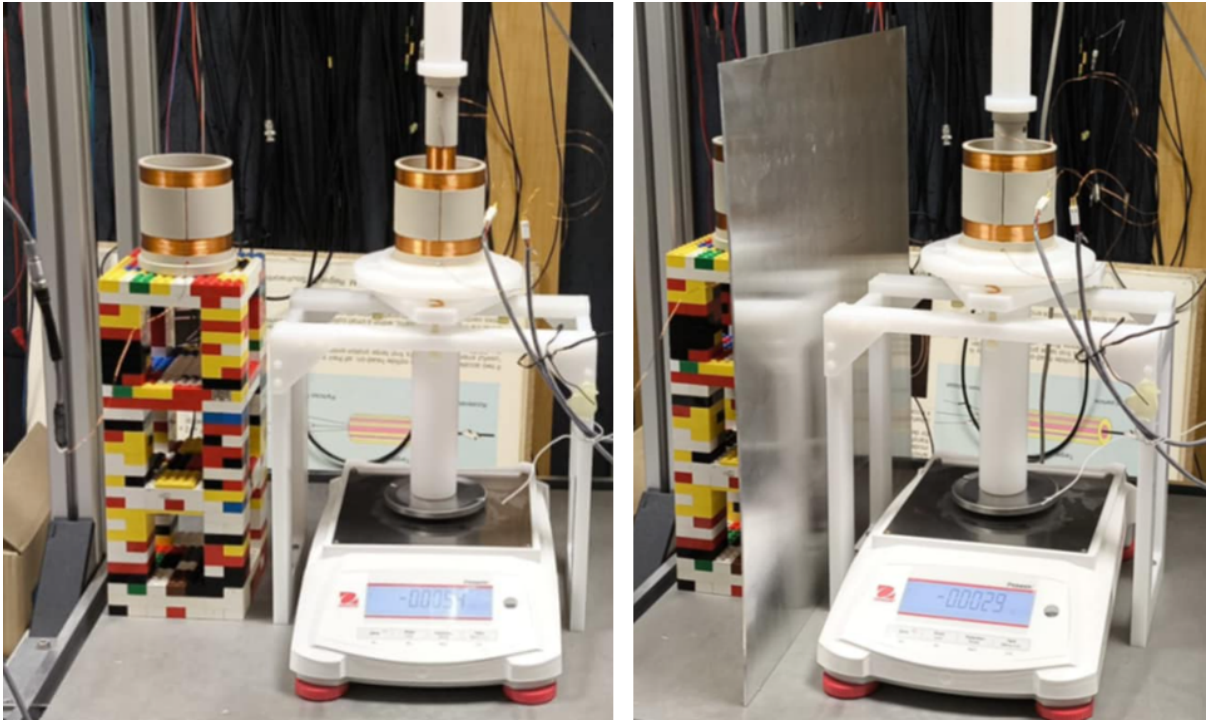
Figure 2.11: Left: two RLVDT's, one on the main suspension and one on the LEGO ® -suspension Right: two RLVDT's separated by an aluminum sheet [20]
