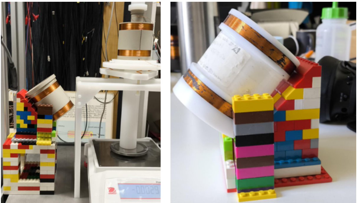
Figure 2.12: Left: two RLVDT's, one on the main suspension and one in the angle holder Right: detailed picture of outer coils in the angle holder [20]
