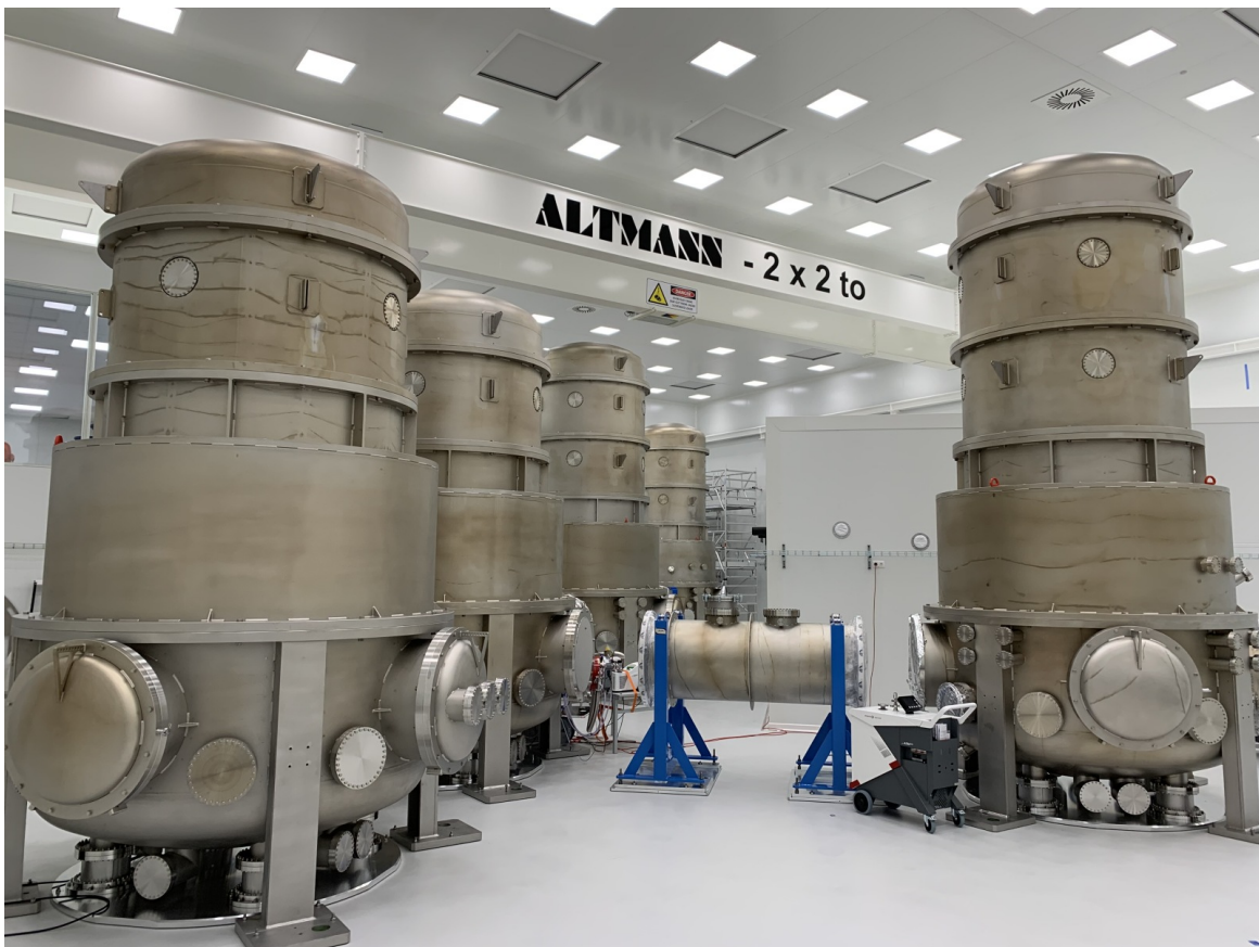
FIGURE B.1: Picture showing the construction of the interferometer. Each tower will contain suspended optics and measurement equipment [27].
