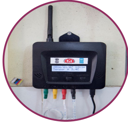
Temperature Logger TL for accurate remote temperature monitoring in real time
