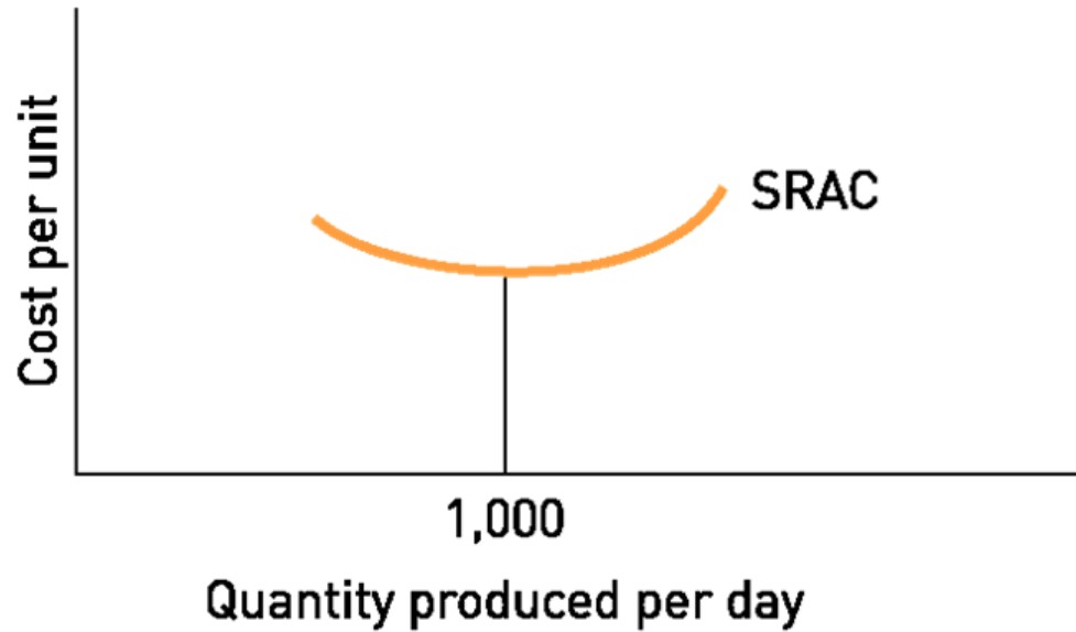
(a) Cost behaviour in a fixed-size plant
