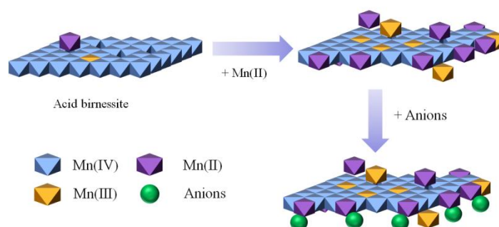
Figure 1: A proposed mechanism for the combined suppressive effects of dissolved Mn(II), pH and naturally occurring anions on the reactivity of nanostructured birnessite.
