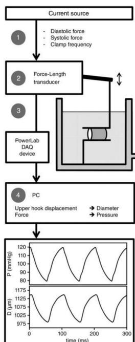
Figure 2. Rodent Oscillatory Tension Set-up for measuring Arterial Compliance (ROTSAC). (Leloup et al, 2016)
