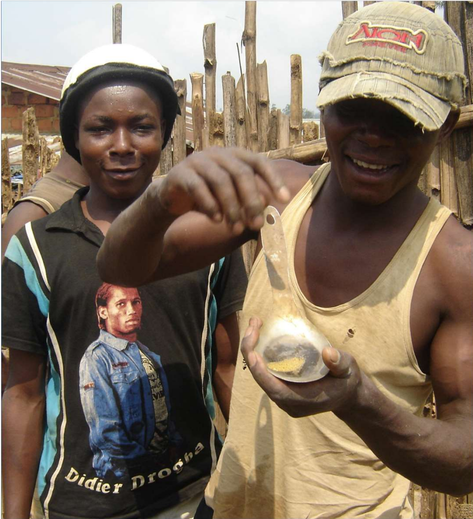
Burning gold with nitric acid Picture: Sara Geenen
