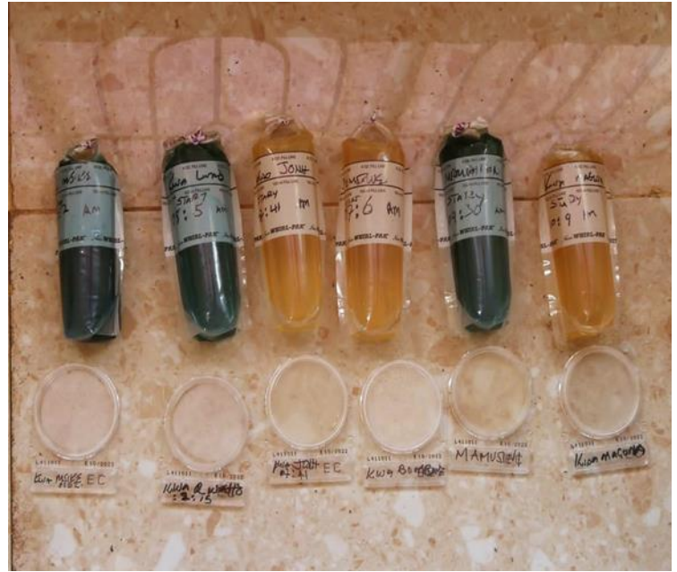
Image 9: Water quality assessment using water sample colour change
