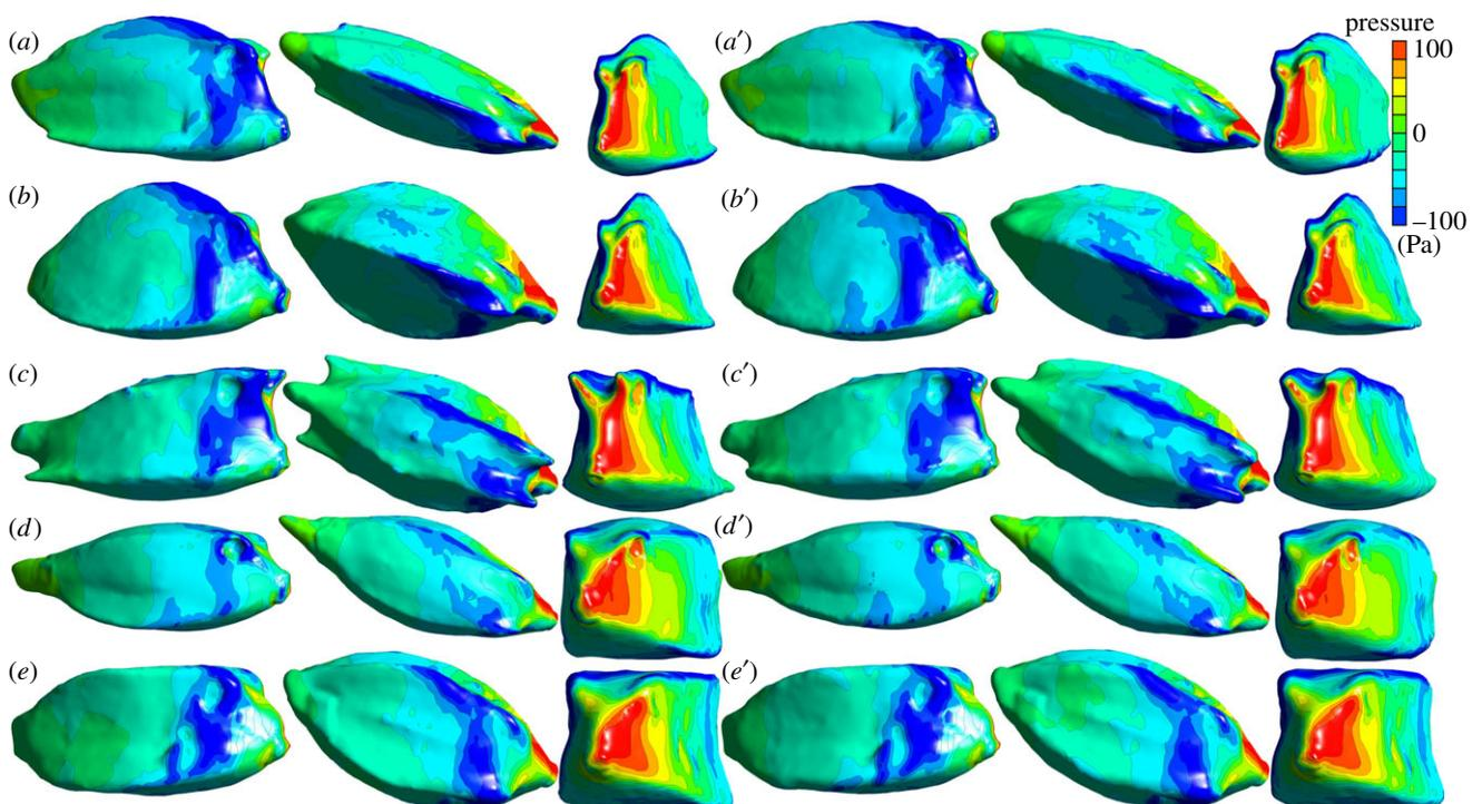
**Figure 5.** Static pressure experienced by the carapaces at a  $-20^\circ$  yaw angle of attack in a water flow of  $0.5 \text{ m s}^{-1}$  as calculated by CFD for the original model of (a) *A. guineensis*, (b) *L. triqueter*, (c) *L. cornuta*, (d) *O. cubicus* and (e) *R. rhinorhynchus*; and (') their corresponding reduced-keel models. From left to right, views are lateral, dorsal and frontal.
