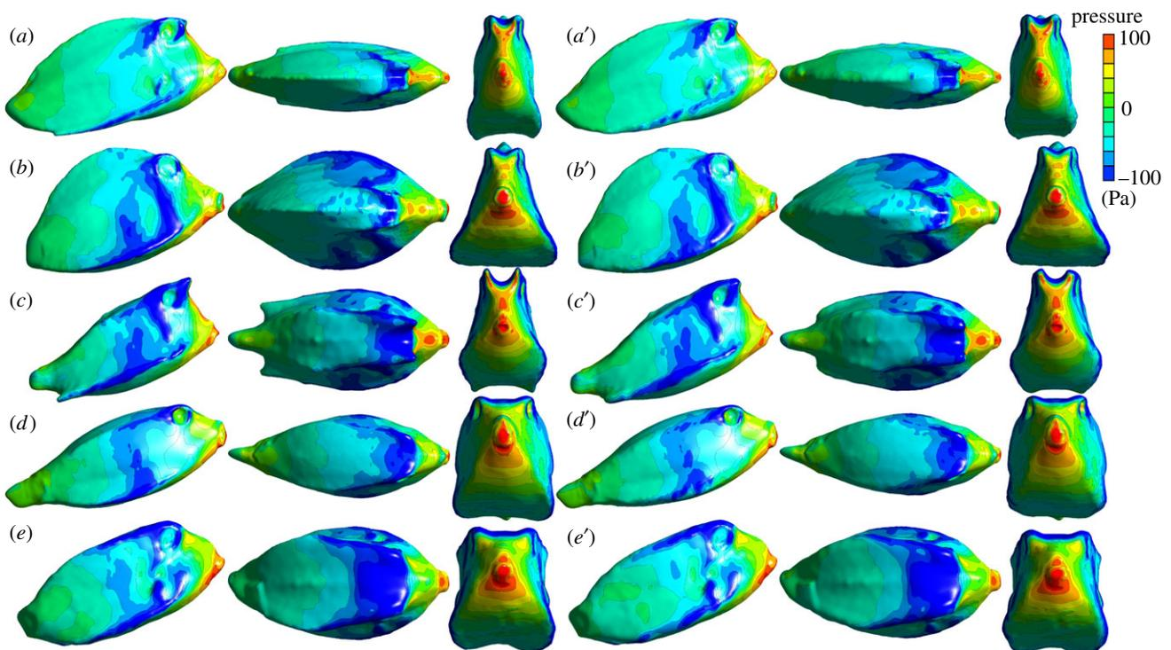
**Figure 4.** Static pressure on the carapaces at a 20° pitch angle of attack in a water flow of 0.5 m s<sup>-1</sup> as calculated by CFD for the original model of (a) *A. guineensis*, (b) *L. triqueter*, (c) *L. cornuta*, (d) *O. cubicus* and (e) *R. rhinorhynchus*; and (') their corresponding reduced-keel models. From left to right, views are lateral, dorsal and frontal.
