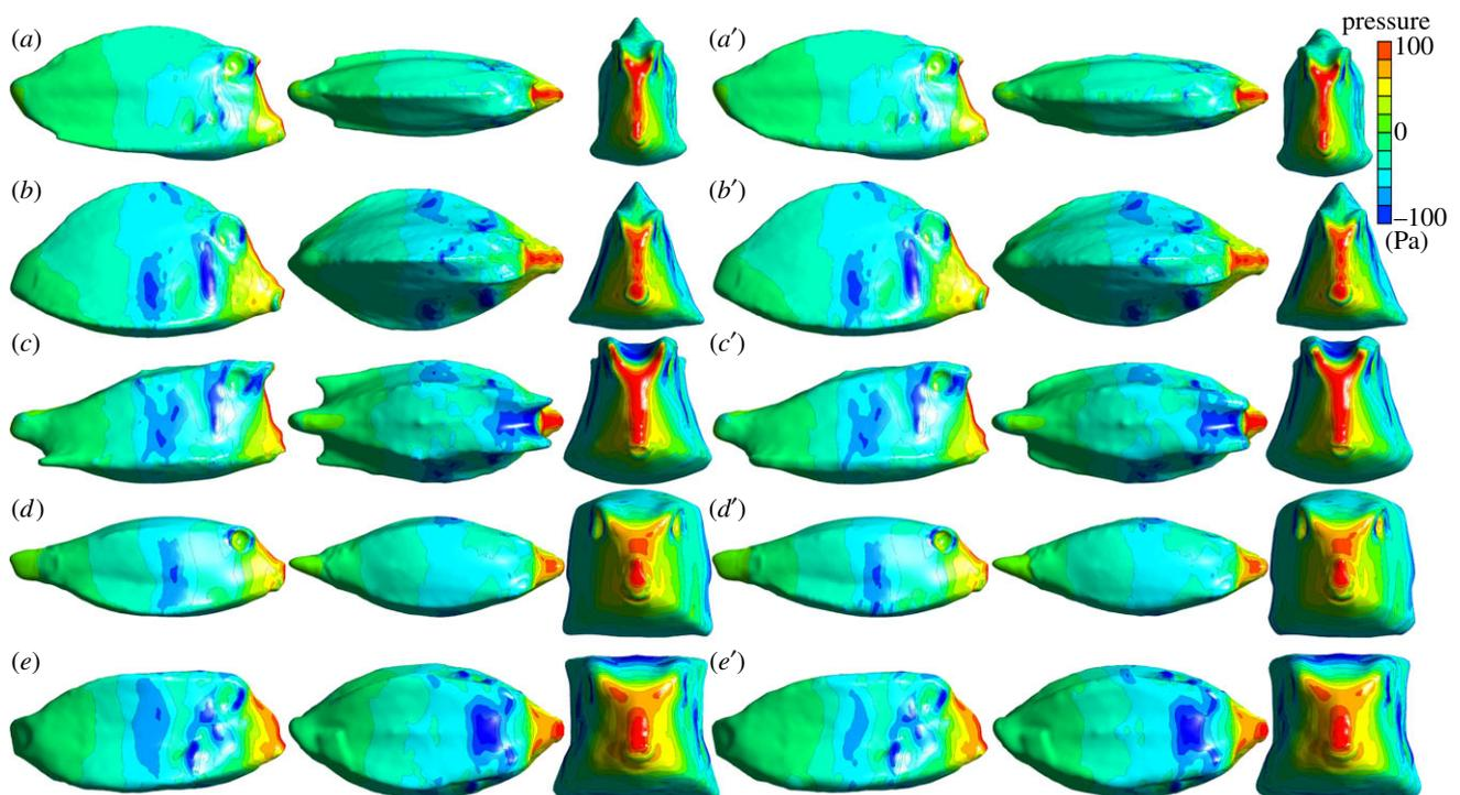
**Figure 3.** Static pressure experienced by the carapaces with their rostro-caudal axis parallel to a water flow of  $0.5 \text{ m s}^{-1}$  as calculated by CFD for the original model of (a) *A. guineensis*, (b) *L. triqueter*, (c) *L. cornuta*, (d) *O. cubicus* and (e) *R. rhinorhynchus*; and (') their corresponding reduced-keel models. From left to right, views are lateral, dorsal and frontal.
