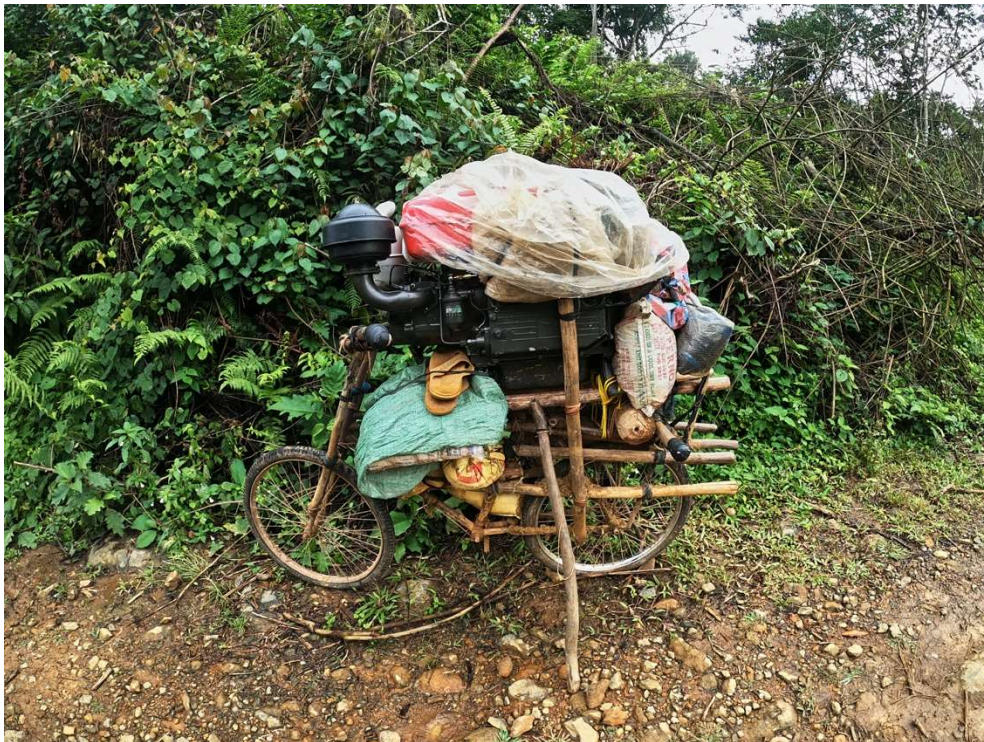
Moto pump charged to a modified bike (Credit: Simon Marijsse)
